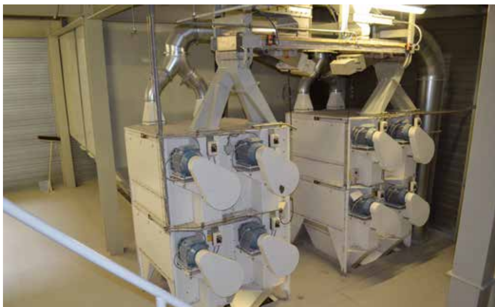
The brushing machines give the grains a shiny appearance.
