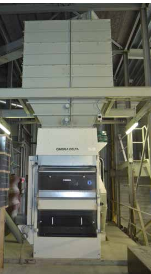
This cleaner thoroughly cleans the grains and seeds upon delivery and removes dust particles. The state-of-the-art machine can thoroughly clean and dust twenty tons per hour.
