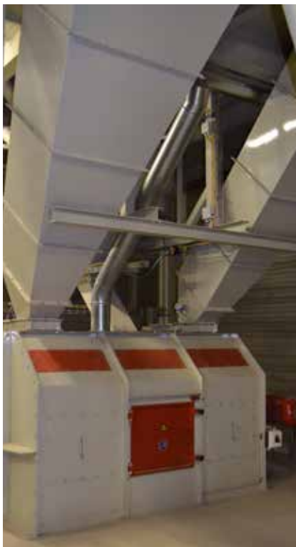
The new mixers ensure a homogeneous composition of each mixture, making sure each mixture has a balanced amount of different grains and seeds.
