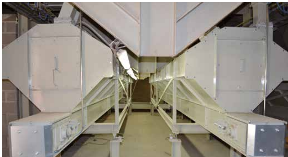
These are two of a total of five silo scales which weigh the individual ingredients of each mixture, as stipulated by the production instructions. It allows us to measure out each mixture with extreme precision.
