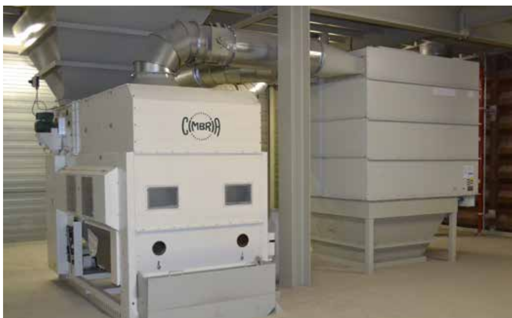
In this secondary cleaner the grain mixtures and seeds are thoroughly cleaned and dusted a second time, just before they are being packaged.
